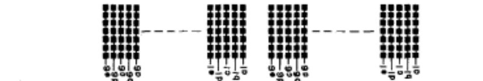
Waveform for displaying a 0 on the most significant digit.
