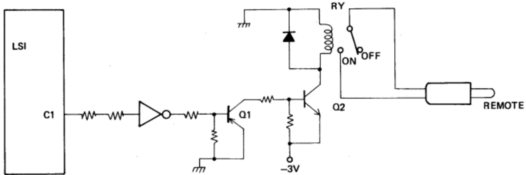
When signal C1 is HIGH, transistors Q1 and Q2 turn on causing relay RY to be switched on so that the REMOTE terminal becomes active.
