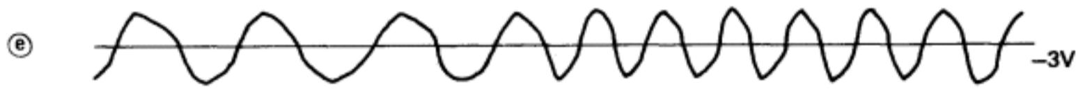
Data output C2 from the LSI is integrated (waveform **d**) and shaped into an AC waveform (waveform **e**) by capacitor c1 and resistor r1.
