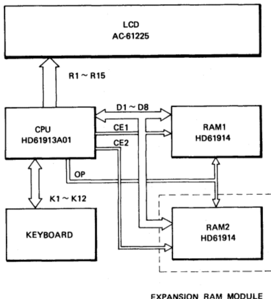
**LCD:** 12-digit dot-matrix display. A character or a number is displayed in  $5 \times 7$  dots.
